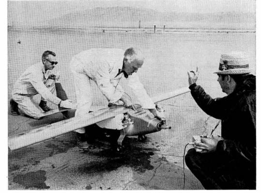
ABOVE ROAR of three motors going full blast, Ted White (right) signals that the synchronization of the engines sounds OK. Dan Parsons (7214), center, adjusts the needle valves while Chad Miller (7214) anchors the Beast. The radio-controlled plane is being used to drop 12-pound test units.
